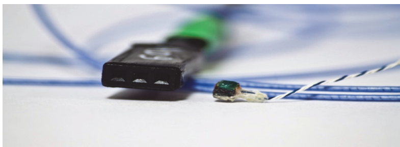
Fig. 2. A HQ220-L165-S sensor. Source: own work
