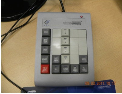
Photo 4 The device controlling the communication between computer stations
